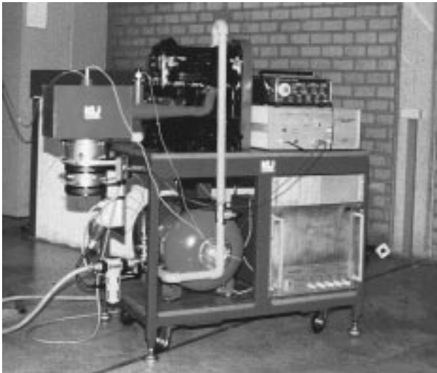
figure 11: The experimental setup of the active silencer on the exhaust of the cold engine simulator.
