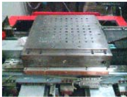
Figure 5: A xy feed table with three linear drives for high speed milling application
