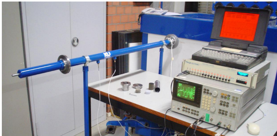
Figure 5: Laboratory setup for acoustic impedance measurement.
